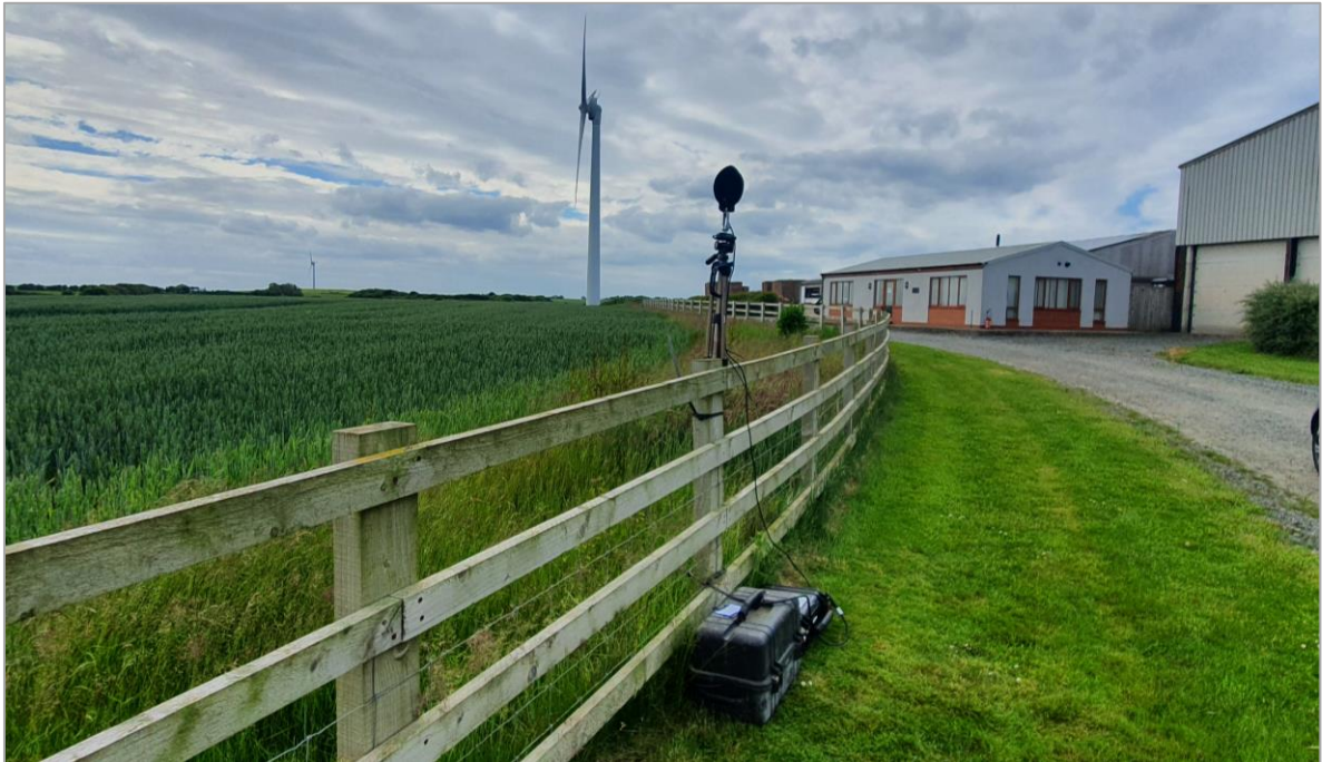
Figure 3.6 – Noise monitoring installations at Position P2 – view facing north-west
